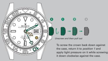
After every use, carefully screw the crown back down against the case to guarantee the waterproofness. The crown should never be unscrewed under water.
