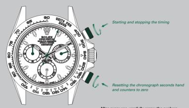
After every use, carefully screw the pushers back down against the case to guarantee the waterproofness. The pushers should never be unscrewed under water.
