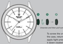
To screw the crown back down against the case, return it to *position 1* and apply light pressure on it while screwing it down clockwise against the case.
