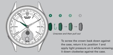
After every use, carefully screw the crown back down against the case to guarantee the waterproofness. The crown should never be unscrewed under water.
